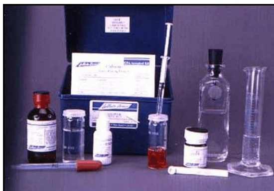
Figure 39. Test kit for checking “free” chlorine in a solution.
